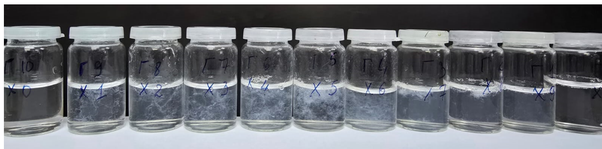
Fig. 1. Formation of chitosan-gellan PECs depending on volume ratio of interacting components
